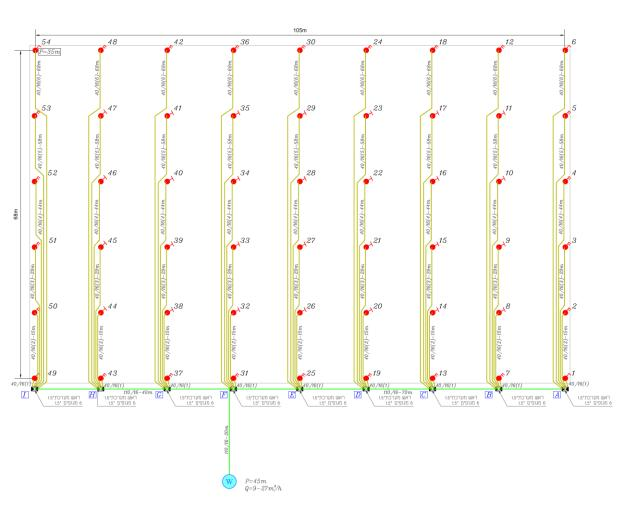
Sprinkler distances are determined according to the specific design requirements. Among the various design determine parameters, we consider the soil structure and composition, the type of grass, the wind regime and the shading created by the stadium structure.
